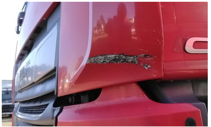
4: Screen Front Chipped Over 10mm
